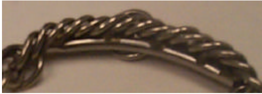
ILLEGAL – has round bar welded on the inside of the chain.
